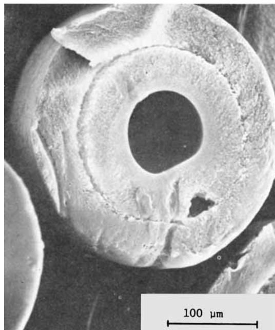
Fig. 7. Concentric split hollow fiber—"fiber within a fiber." Spinning formulation, PS/PVP/DMA = 31/15/54; viscosity, 76,000 cP; bore precipitant, DMA/water = 3/1; jet temp., 52°C ( L_p = 6 cm/sec atm).
